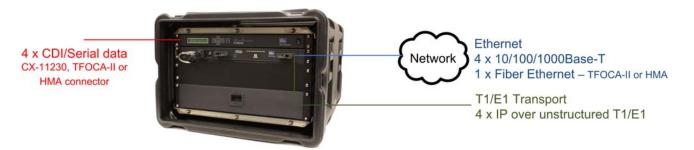
Ethernet and CDI/Serial data may be user or network side connections. T1/E1 is a network side connection only.
